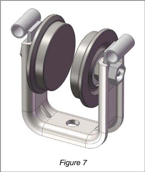
Figure 7 Figure 7 shows Collector Mounting Brackets, #10-2125-00 (bracket is attached under the wheel axle bolt), typical for 2T-750-2, 3T-1150-4, 3T-750-2 and 3T-1150-4 that use this stamped steel yoke.
