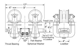
**Note** Loadbar does not accept a motorized trolley—use drive tractor.
