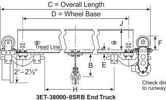
Check dimension "F" and "J" for clearance to runway and suspension.
