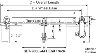
Check dimension "F" and "J" for clearance to runway and suspension.
