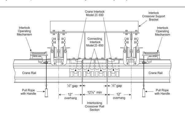
Interlocking Cranes to Crossover (Typical) Shown with 2I-930 Crane Interlocks and 2I-850 Connecting Interlocks with Side Contact Conductor Bars on the Cranes and Crossover.
