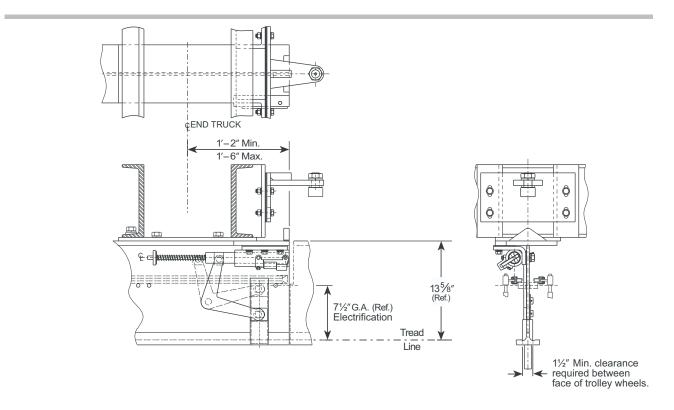
**3I-10A Connecting Interlock** Manual Operation, Shown in Crane Bridge without Step Cut, with Side Contact Conductors
