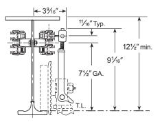
Trolleys with 5" Dia. Wheels, Trolley Mounted Collector Minimum Rail Depth Req'd: 3RH13-30,3RH13-36
