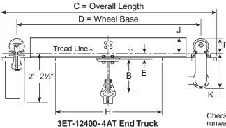
Check dimension "F" and "J" for clearance runway and suspension.
