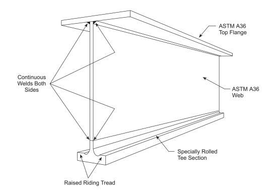
TC/American "450" Series Patented Track Rail is a 3-piece composite beam consisting of an ASTM A36 Top Flange, ASTM A36 Web and a load carrying Tee Section rolled from high carbon-manganese alloy steel. The Tee Section is  $4\frac{1}{2}$ " wide with a raised riding tread.
