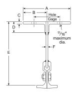
Maximum load <u>per trolley wheel</u> for all "200" Series Rail is 1000 pounds (2,000 lbs. per two-wheel trolley).
