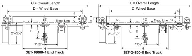
Check dimension "F" and "J" for clearance to runway and suspension.
