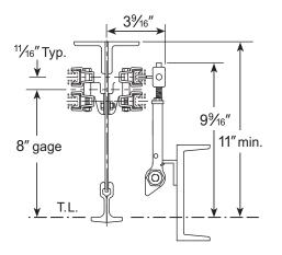
**Crane Runways** Trolleys with 3", 4" and 5½" Dia. Wheels, End Truck Mounted Collector Minimum Rail Depth Req'd: 2GR11-16
