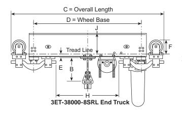
Check dimension "F" and "J" for clearance to runway and suspension.
