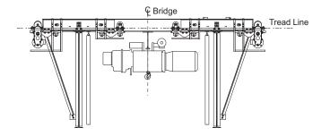
Typical Truss Crane, Single Girder, Double Truss
