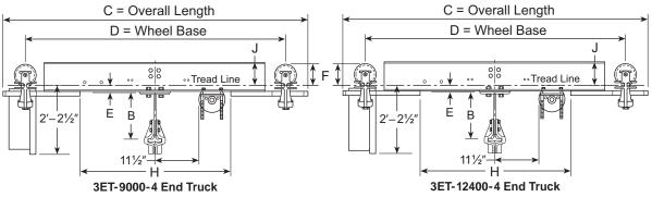
Check dimension "F" and "J" for clearance to runway and suspension.
