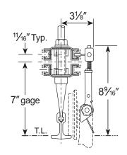
**Monorails** Trolleys with 3" and 4" Dia. Wheels, Trolley Mounted Collector
