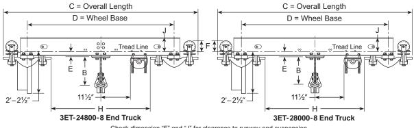
Check dimension "F" and "J" for clearance to runway and suspension.
