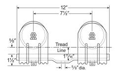
Consists of two 2T-850-2 trolleys coupled by LB-155-1 Loadbar.
