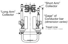
Typical Web Mounted Conductor Bar with Side Contact Collectors
