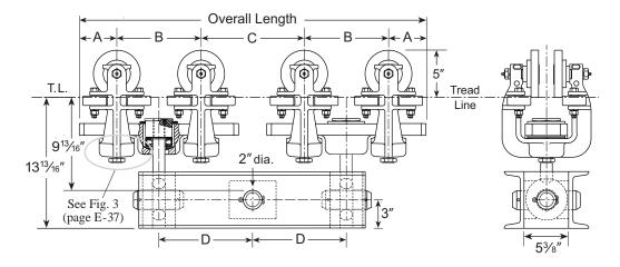
3T-24800-8SR consists of two Model 3T-12400-4SR trolleys coupled by a fabricated loadbar with a hook bearing.
