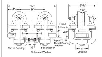
**Note** Loadbar does not accept a motorized trolley—use drivetractor.
