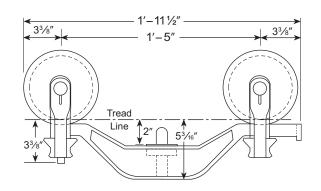
Consists of two 2T-3000-2 trolleys coupled by LB-519 Loadbar.
