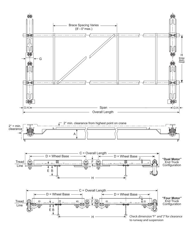
**Double Girder Crane Clearance Drawing**
