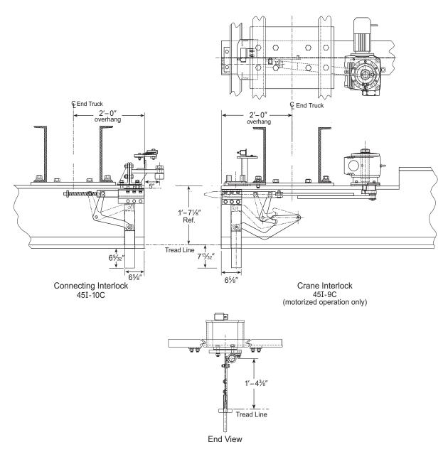
**Crane to Crane Interlock Shown**
