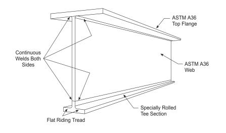
TC/American "400" Series Railmaster II Patented Track Rail is a 3-piece composite beam consisting of an ASTM A36 Top Flange, ASTM A36 Web and a load carrying Tee Section rolled from high carbonmanganese alloy steel. The Tee Section is 4<sup>1</sup>/<sub>16</sub>" wide with a flat riding tread.
