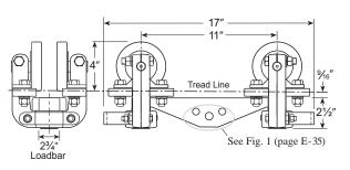
Consists of two Model 2T-2000-2 trolleys coupled by an LB-167 Loadbar with Hook Bearing or Swivel Bushing.
