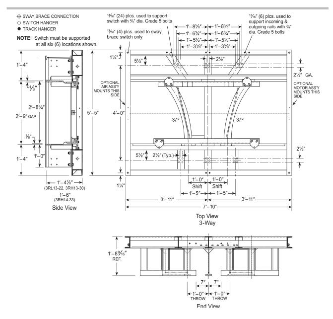
**Note** Maximum load on all switches is 14,000 lbs. (limited to 1250 lbs./wheel for "L" Series Rail; 3500 lbs./wheel for "H" Series Rail).
