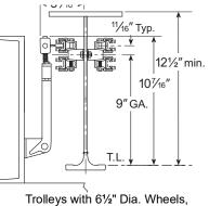
Trolleys with 6<sup>1</sup>/<sub>2</sub>" Dia. Wheels, End Truck Frame Mounted Collector Minimum Rail Depth Req'd: 3RH13-30, 3RH13-36
