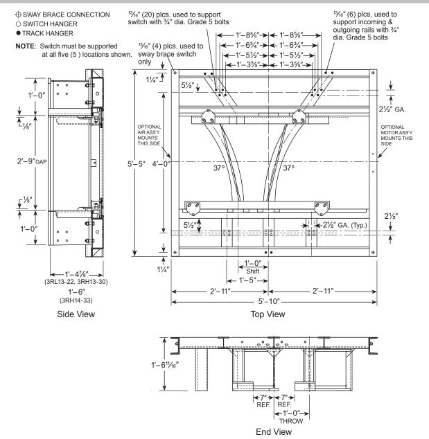
**Note** Maximum load on all switches is 14,000 lbs. (limited to 1250 lbs./wheel for "L" Series Rail; 3500 lbs./wheel for "H" Series Rail).
