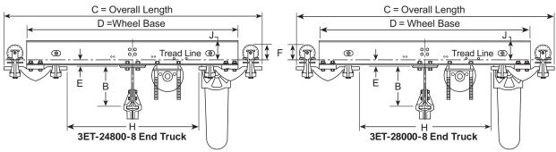
Check dimension "F" and "J" for clearance to runway and suspension.
