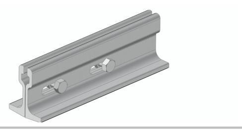
The assembled 2R3-5T rail is made of twin sections bolted together back-to-back to form a solid unit. The exceptional strength of the rail is due to the design, high quality of steel, lap splice and the added strength provided by hangers. The rail has a balanced section, the head of the rail being a mass of steel equaling the weight of the flanges.
