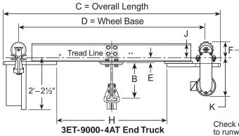
Check dimension "F" and "J" for clearance to runway and suspension.
