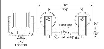
Consists of two 3T-750-2 trolleys coupled by an LB-155-1 Loadbar.
