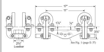
Consists of two Model 3T-2000-2SR trolleys coupled by an LB-167 Loadbar.
