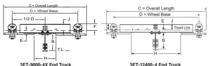
3ET-9000-4X End Truck 3ET-12400-4 End Tru Check dimension "F" for clearance to runway and suspension.
