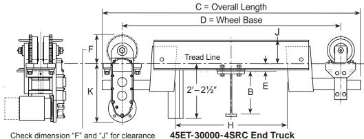
Check dimension "F" and "J" for clearance to runway and suspension.
