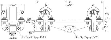
Consists of two Model 3T-2000-2SR trolleys coupled by an LB-212 Loadbar.
