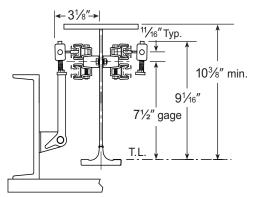
**3" and 4½" Wheel** Trolleys with 3" and 4½" Dia. Wheels, End Truck Frame Mounted Collector Minimum Rail Depth Req'd: 3RL11-19,3RL11-21
