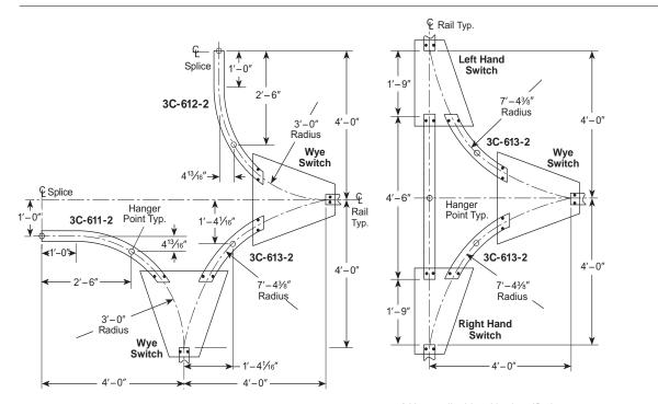
\* Not applicable with electrified switches due to phase reversal
