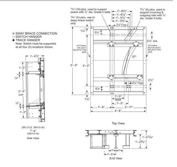
**Note** Notes:Maximum load on all switches is 14,000 lbs. (limited to 1250 lbs./wheel for "L" Series Rail; 3500 lbs./wheel for "H" Series Rail).
