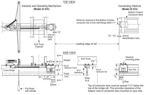
Bottom Contact Electrification (or Non-Electrified)
