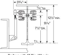
Trolleys with 5" Dia. Wheels, End Truck Frame Mounted Collector Minimum Rail Depth Req'd: 3RH13-30,3RH13-36
