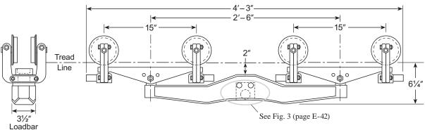
Consists of two Model 2T-3100-4 trolleys with Swivel Bushings, coupled by an LB-215 Loadbar.
