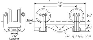
Consists of two Model 2T-2000-2SR trolleys coupled by an LB-167 Loadbar with Hook Bearing or Swivel Bushing.
