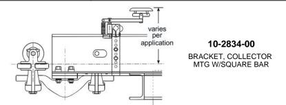
Typical Bottom Contact Collector Mounting (shown on crane end truck or hoist carrier)
