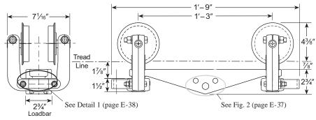
Consists of two Model 3T-2000-2 trolleys coupled by an LB-212 Loadbar.
