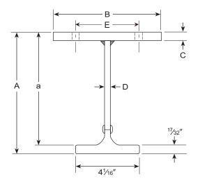
Maximum load <u>per trolley wheel</u> for all "400" Series rail is 2600 pounds (5200 lbs. per two-wheel trolley), based upon "Square Cut" ends. For higher wheel loads or to match existing rails, contact the factory for information about addition of a Tension Strip welded under the tee section which allows the maximum load per trolley wheel to be increased up to 3300 pounds (6600 pounds per two-wheel trolley).
