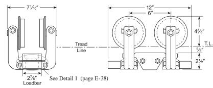
Consists of two Model 3T-2000-2 trolleys coupled by an LB-114 Loadbar.
