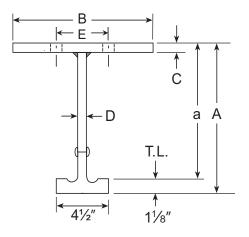
Maximum load <u>per trolley wheel</u> for all "450" Series rail is 9000 pounds (18000 lbs. per two-wheel trolley), based upon "Square Cut" ends.
