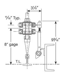
**Crane Runways** Trolleys with 3", 4" and 5½" Dia. Wheels, End Truck Frame Mounted Collector
