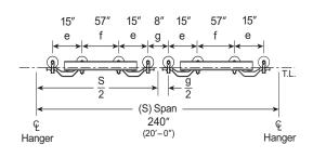
Step 5 Select Rail Size from Rail Load Tables in Rail Section of TC/American Systems Catalog
