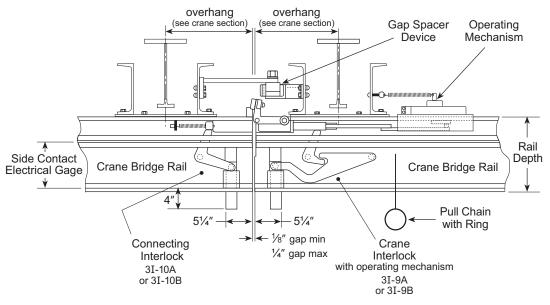
Interlocking Crane to Crane (325 "H" Series)
