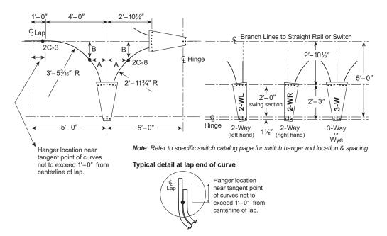
Typical Layout for Standard Radius Curves, Non-Electrified Tongue Switches
