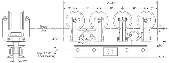
Consists of two Model 2T-3100-4CC trolleys, coupled by an LB-126-1 Loadbar.
