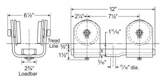
Consists of two 3T-850-2 trolleys coupled by an LB-155-1 Loadbar.
