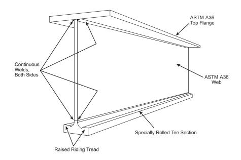
TC/American "325L" and "325H" Series Patented Track Rails are 3-piece composite beams consisting of an ASTM A36 Top Flange, ASTM A36 Web and a load carrying Tee Section rolled from high carbonmanganese alloy steel. All 325 Series Tee Sections are 3<sup>1</sup>/<sub>4</sub>" wide with a raised riding tread. The 325L Tee Section is <sup>7</sup>/<sub>16</sub>" thick, measured at the riding tread; the 325H Tee Section is <sup>11</sup>/<sub>16</sub>" thick.
