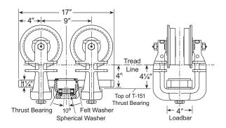
**Note** Loadbar does not accept a motorized trolley—use drivetractor.
