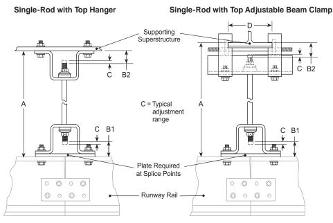
$\label{eq:Hanger Rod Length = A - (B1 + B2)} \\ \mbox{Dimension C = typical adjustment at each end of hanger rod}$
