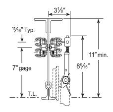
Monorails and Bridges Trolleys with 3" and 4" Dia. Wheels, Trolley Mounted Collector Minimum Rail Depth Req'd: 2GR11-16
