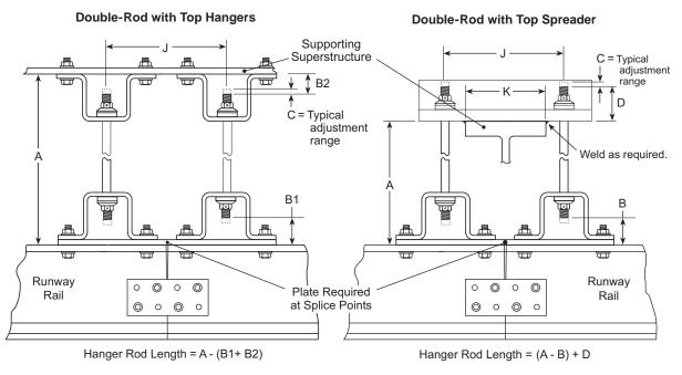
Adjust hanger rods so that load is carried equally on each rod.
