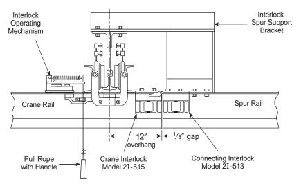
Interlocking Cranes to Spur Rail (Typical)
