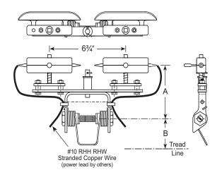
Shown are two 10-2125-00 Collector Mounting Brackets installed on a 2T-750-2 Trolley (bracket bolts to trolley yoke under the axle bolt). Order one bracket for each collector to be mounted on 2T-750-2, 2T-1150-4, 3T-750-2 and 3T-1150-4 Trolleys.
