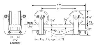
Consists of two Model 3T-2000-2 trolleys coupled by an LB-167 Loadbar.
