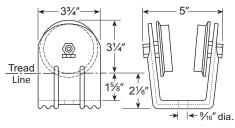
**Note** Model 2T-850-2C is the same as Model 2T-850-2 except it has an 11/16" diameter hole in the yoke for use with crane end trucks.
