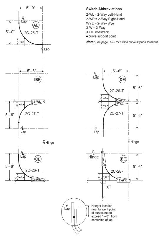
Typical detail at lap end of curve
