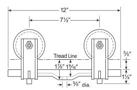
Consists of two 2T-750-2 trolleys coupled by LB-155-1 Loadbar.
