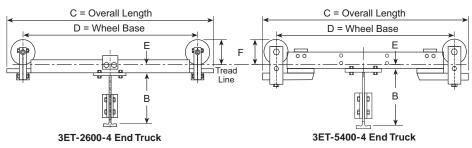
Check dimension "F" for clearance to runway and suspension.
