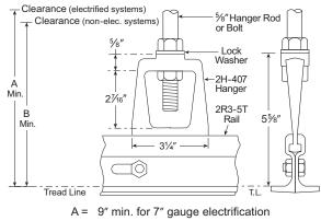
A =  $10^{"}$  min. for  $8^{"}$  gauge electrification
