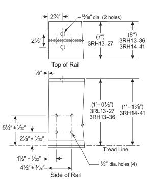
**Note** For all 2000 Series Switches, order #10-2374-00 Splice Plate Assembly for each switch to curve or switch to straight rail connection.
