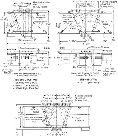
2'-11<sup>3</sup>/16" 5'-103/8' Electric Junction Box 1" Shimming Allowance 6 x 8 x 3¾" NEMA 12 B.O.S 9¾"--1-1-8 11/₄"→ 31/8' Ref. R 4 1'--1% 7% GA Tread Line I 4¾ Clearance Δ 8" Shift 8" Shift Pull Rope Shown with Standard (4) Bar S.C. **Channel Electrification** 3ES-697-2 Three-Way
